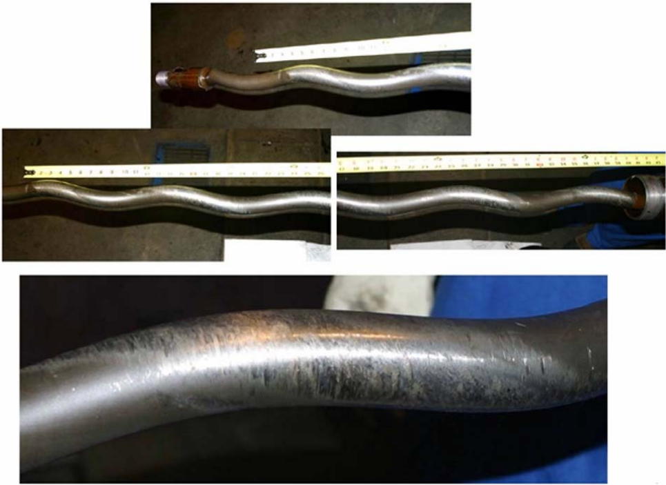
Figure 6.22 KUDU - Images of Rotor Condition at the Discharge End
