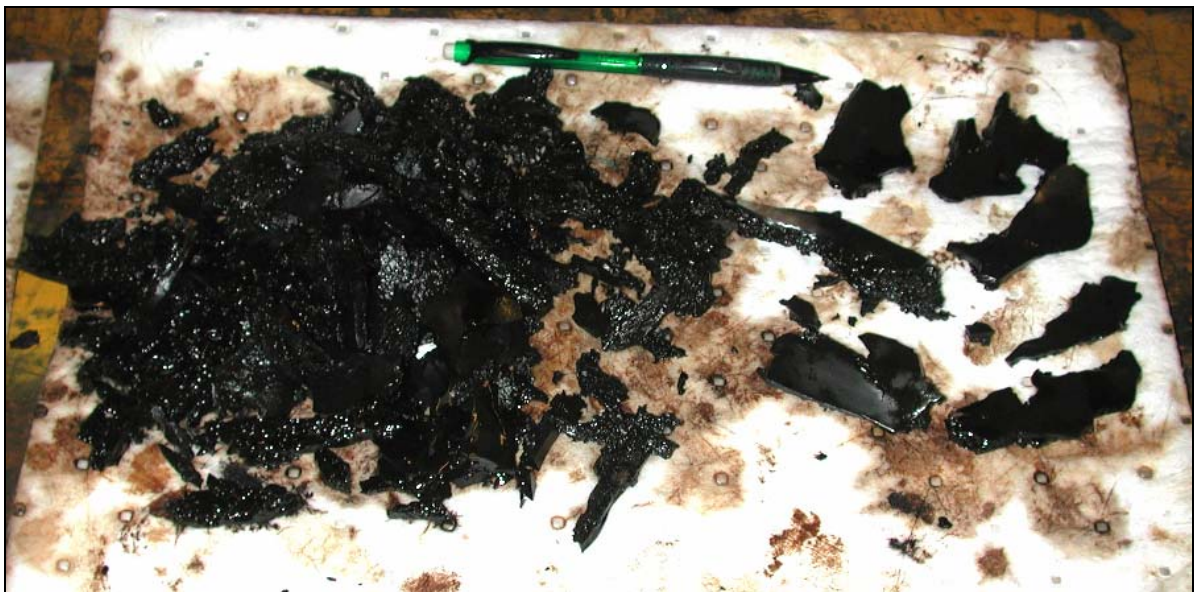
Figure 4.20 Netzsch - Elastomer Material Found in the Strainer after Testing with 100% Oil
